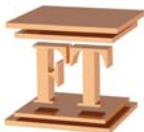
SOLID-METAL THERMAL COLUMNS IN CONVENTIONAL PCBs
