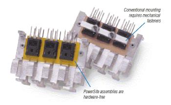
The improvement in thermal transfer with PowerSites is most beneficial in power electronics application with high thermal demands. Reduction in device operating temperature is as high as  $2^{\circ}$ C/W of dissipated heat for a TO-220 and  $1^{\circ}$ C/W for a TO-247. With the elimination of attachment hardware, PowerSites have no pressure dependency, reduce SKUs, and allow the placement of other PCB components closer to the heat sink subassembly (UL clearance to 'ground').
