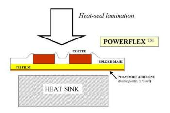
The Kapton\* MT substrate and thin coating of polyimide adhesive of the proprietary TPI bond film yield a construction where the copper conductors are bonded within about 1.3 mils of the heat sink (thermal impedance of about  $0.1^{\circ}\text{C-in}^2/\text{W}$ ), while providing over 4000v dielectric strength.
